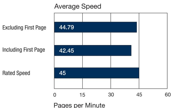
Print speed is tested using BLI's Monochrome Test Original with 6% page coverage. The test page is printed in a quantity equal to double the vendor's rated print speed for the device in each mode tested (e.g., if the vendor's rated print speed is 20 ppm, 40 pages are printed). The unit was tested using the PCL driver.
