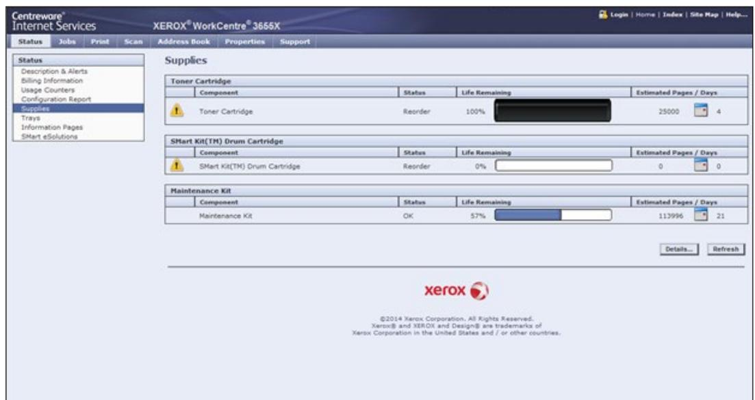
Consumables status for toner, the drum and the maintenance kit are presented in gauges with the percent in text. For paper levels, users must navigate to the trays page, where the status of all paper sources-input and output-is indicated in text. (U.S. model pictured)
