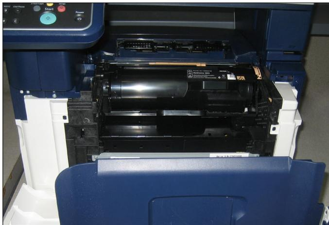
Replacing toner is clean. Users must first turn the control panel to the left and can then open the front cover, which includes most of the output tray; the black tabs on the cartridge must be unlocked, after which users can simply pull out the cartridge. Instructions on the touchscreen and the packaging provide guidance, should it be needed. (U.S. model pictured)
