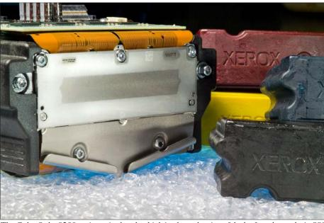
The ColorQube 9200 series print head, which is about the size of deck of cards, packs in 880 nozzles, twice the number per linear inch compared to prior print heads. This enables the head to print 85 pages per minute using molten solid ink. Development of the minuscule nozzles, each only 37.5 microns wide, is considered a major achievement because they deliver higher flow rates—150 million drops of ink per second—despite their reduced size.
