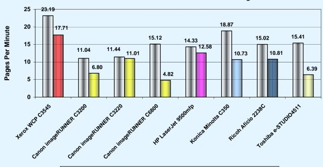
Black-and-White Bars: Test results with the BLI suite run in Mono Mode. Colored Bars: Test results with the BLI suite run in Mono/Color Mode.
