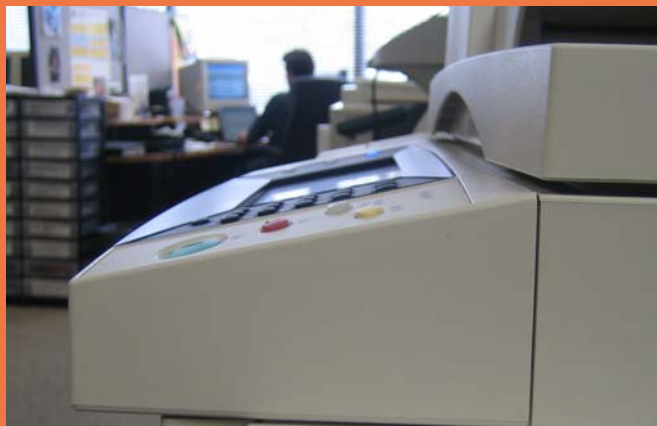
Providing an adjustable tilting control panel would provide users who are physically challenged with easy access to view and use functions on the control panel.
