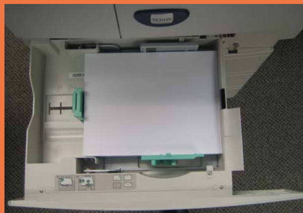
The standard main paper tray supports up to 8.5" x 14" paper size and up to 32 lb. Bond/120gsm paper weight.
