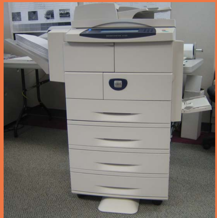
The Xerox WorkCentre 4150 with three optional paper trays, staple finisher, network scanning, and Fax Kit installed.
