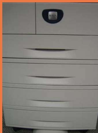
Left: Paper drawers currently have handles that can be grasped from the bottom only. Handles that can also be grasped from the top would make changing the paper size and paper refilling much easier for wheelchair users.
