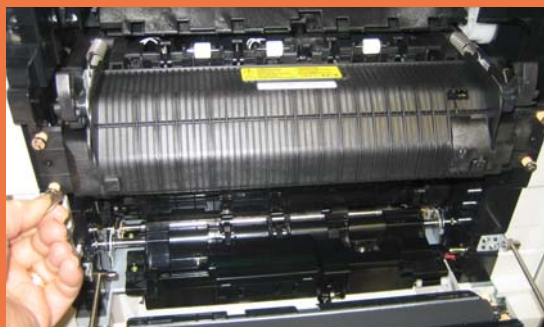
Users can replace most consumables in a matter of minutes. In this case, the BERTL analyst is replacing the fuser unit by turning a couple of screws.
