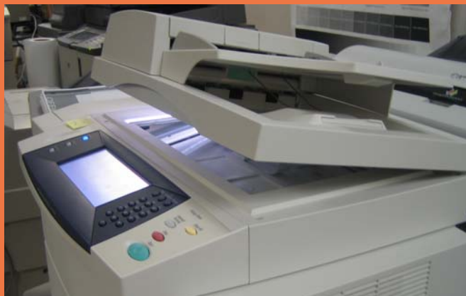
Above: The document feeder can be held open at a low angle aiding platen copying for wheelchair users.
