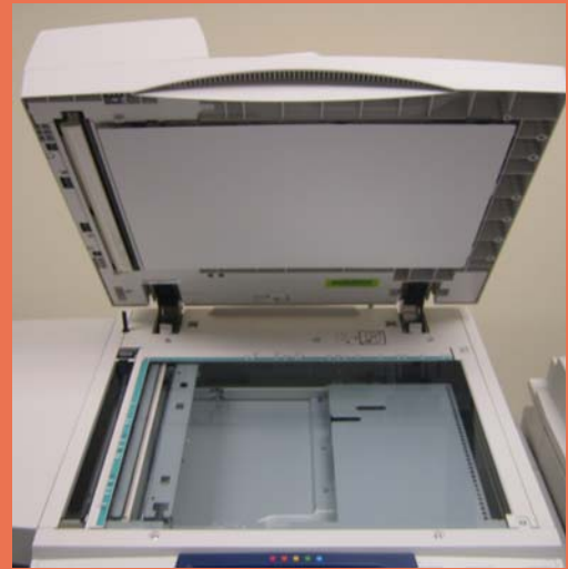
Above and below: The WorkCentre 7435's platen (above) and document feeder (below), with the document feeder's cover opened in order to expose the feeder's misfeed-access area.
