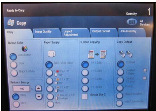
The "Copy" touch screen's main menu provides users with the most common copying choices. The blue bold buttons on the touch screen display currently selected settings.
